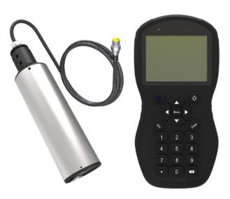
The portable suspended solid(sludge concentration) analyzer consists of a host and a suspension sensor. The sensor is based on a combined infrared absorption scatter ray method, and the ISO 7027 method can be used to continuously and accurately determine the suspended matter (sludge concentration). The suspended matter (sludge concentration) value was determined according to ISO 7027 infrared double scattering light technology without chromatic influence.
