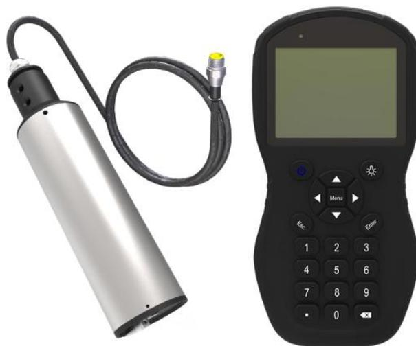
The BOQU portable turbidity meter consists of a host and a turbidity sensor. The turbidity sensor is based on a combined infrared absorption scatter ray method, and the ISO 7027 method can be used to continuously and accurately determine the liquid turbidity. The turbidity value was determined according to ISO 7027 infrared double scattering light technology without chromatic influence.
